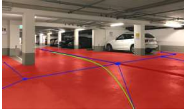
Figure 2: An illustration of the approximated free-space (red) and the road-graph with direction options (blue). Based on the directional choice to go straight, a smooth path can be planned (green) [60].
